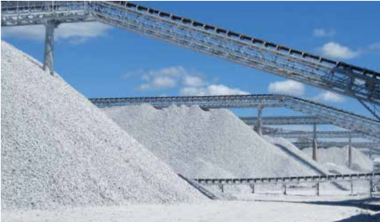
RENOTHERM® is a high calorific refuse-derived fuel made from non-recyclable waste; it is used by a number of industries including cement works
